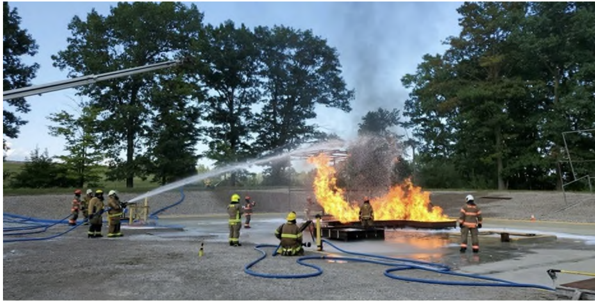
230 ft2 T- pan – Dow test set up
