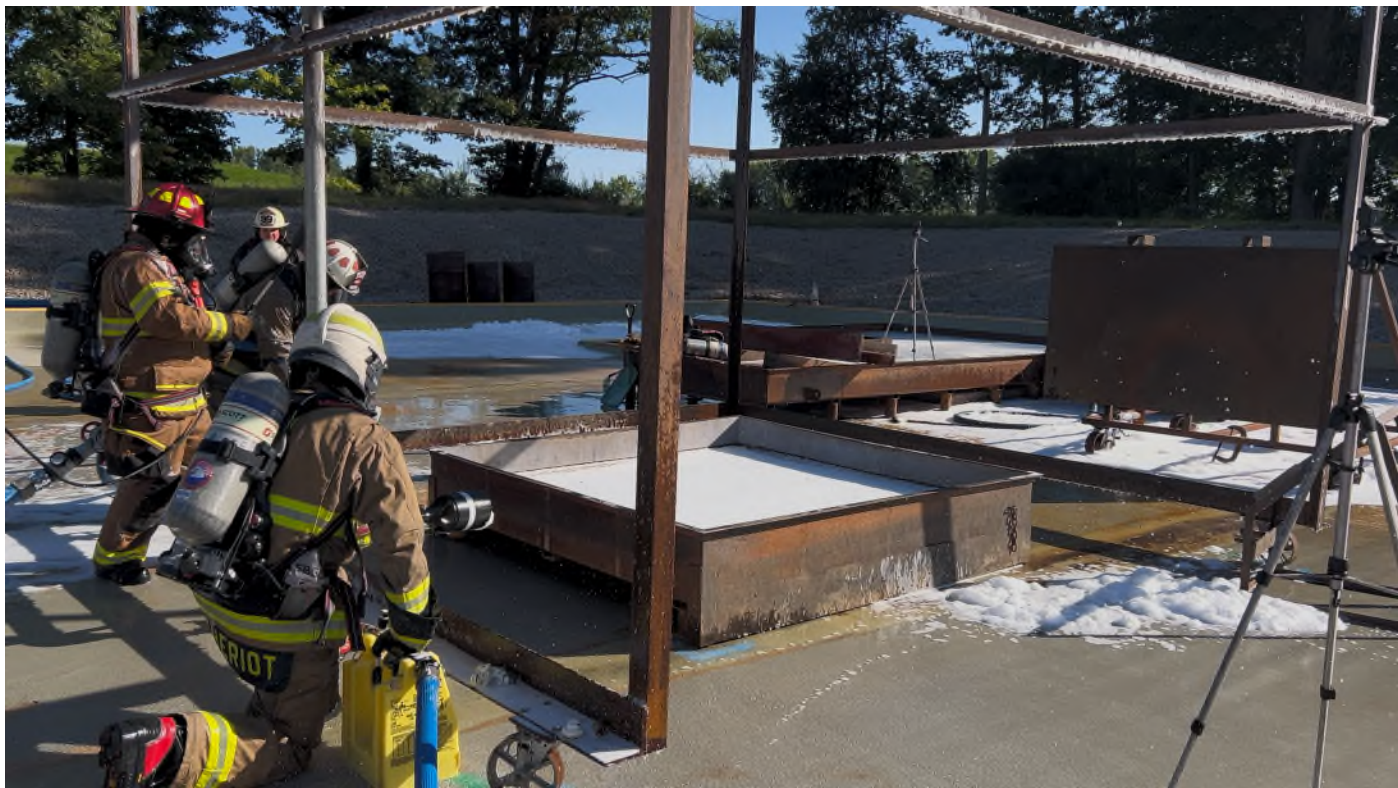
Re-ignition test after extinguishment
