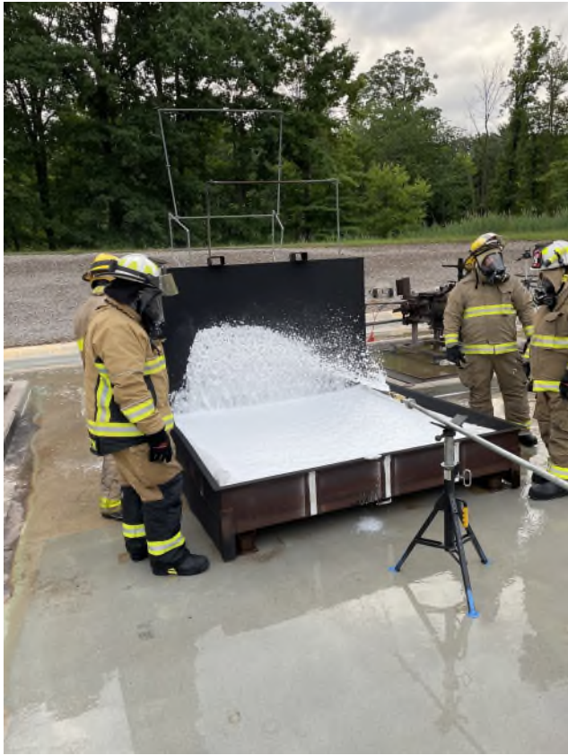
50 ft2 pan – Dow test set up
